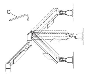
If the monitor is heavier than 4-5 kg, the arm drifts downwards.
